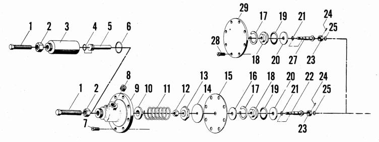
Figure 8-1, Table 8-1 Parts List - Pilot Module
